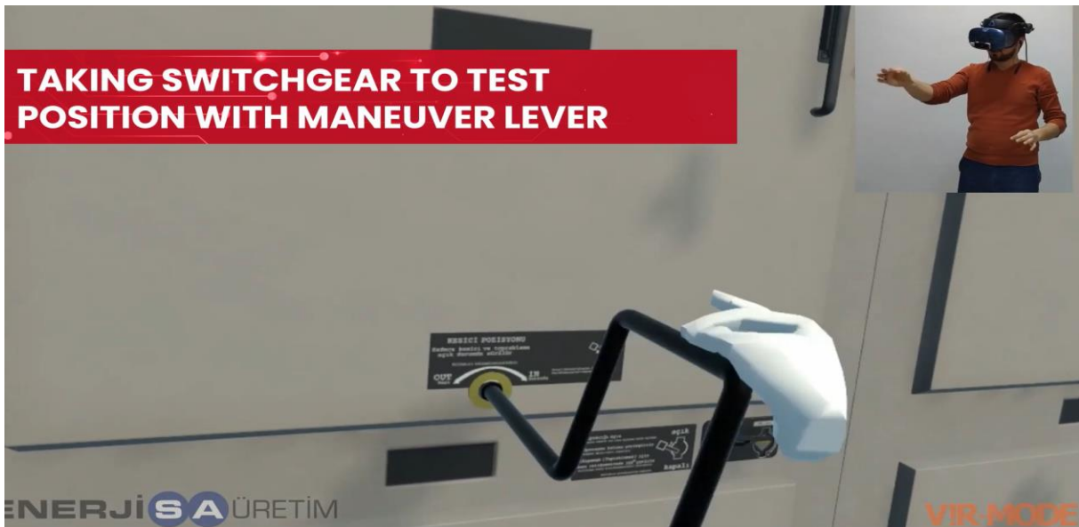
Figure 15. Taking Switchgear to Test Position with Maneuver Lever
