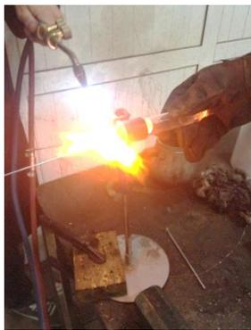
Figure 5. Stage of placement of anode-cathode elements
