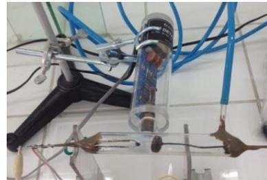
Figure 12. Geiger-Muller counter and X-ray tube
