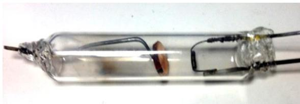
Figure 6. Anode-cathode elements placed in Pyrex glass tube
