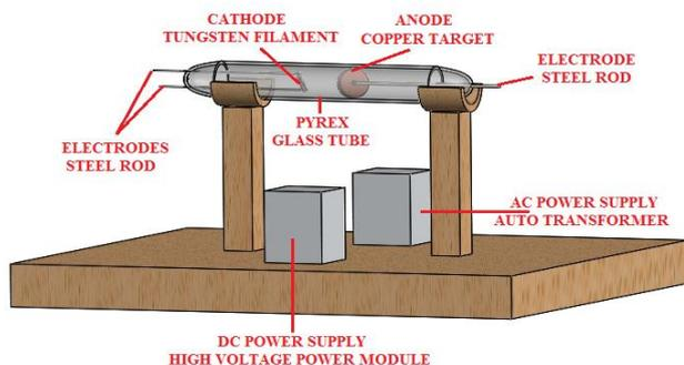
Figure 2. Montage schema of complete system
