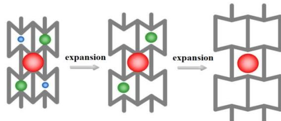
Figure 18. Smart filtering with auxetic feature [66]
