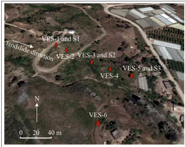
Figure 4. Location of the measurement stations; six vertical electrical sounding (VES-1, VES-2, VES-3, VES-4, VES-5 and VES-6) and three seismic refraction (S1, S2 and S3) stations.
