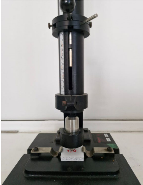
Figure 2. Experimental setup of the Sheen impact drop test used for evaluating impact resistance of Voronoi-core sandwich specimens
