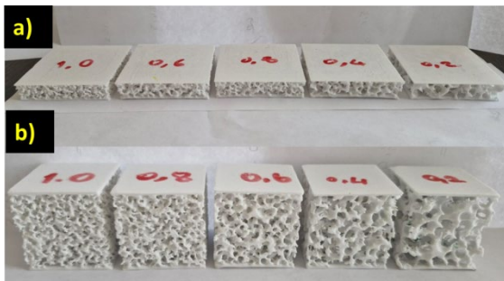
Figure 3. Voronoi-core sandwich specimens prepared for mechanical testing: a) specimens before impact test, b) specimens before compression test
