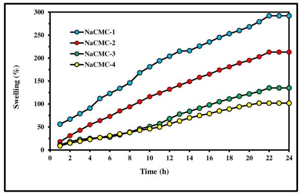
Figure 2. The variation of S% values with time at  $30^{\circ}$ C, pH = 7.0
