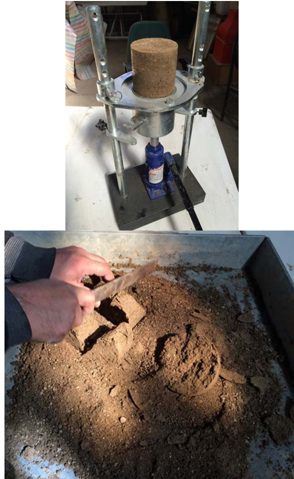
Figure 3. Bringing soil sample out of the mould and its mix with the soil in the plate.
