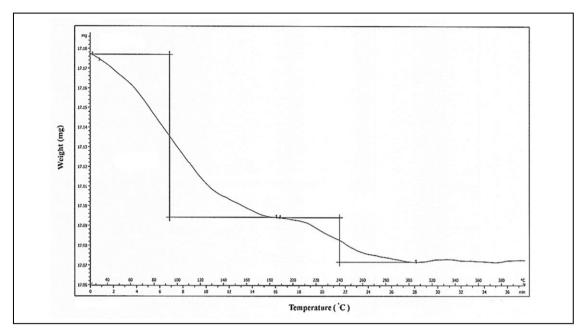
Figure 4. Thermogravimetric analysis curve of chromium doped clay sample
