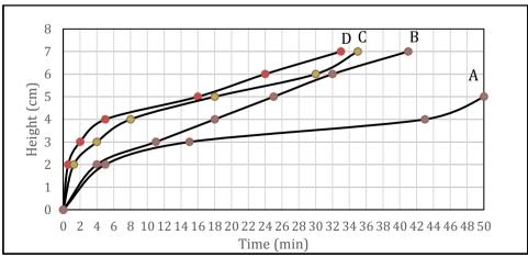
Figure 1. Capillary action curves of (A) natural clay (B) treated clay (C) doped natural clay (D) doped treated clay sample
