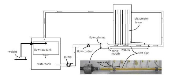
Figure 3. Two dimensional scheme of the experimental set up and test pipe details
