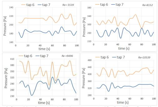
Figure 8. Comparision of pressure variations in pressure taps 6 and 7 at four different Reynolds numbers
