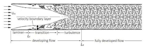
Figure 1. Developing and fully developed flow at pipe entrance
