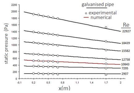
Figure 3. Coparison of numerical and experimental data in terms of pressure variation along the flow
