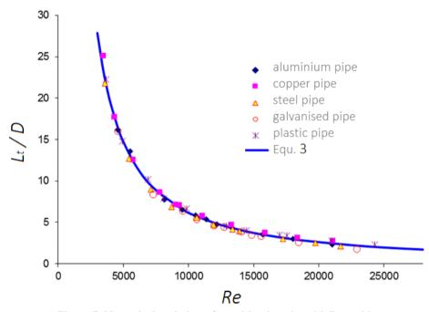
Figure 7. Numerical variation of transition lengths with Reynolds
