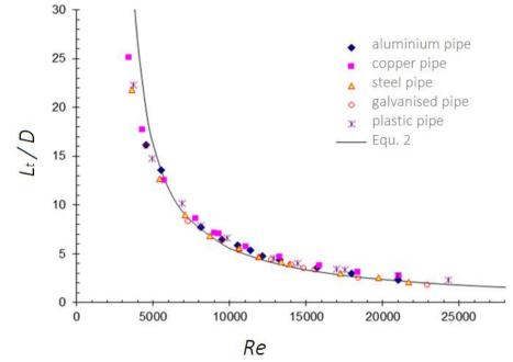
Figure 6. Variation of dimensionless transition lengths with Reynolds
