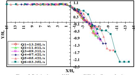
Figure 5. Relation between Y/He versus X/He for all runs of weir (Y/Y  $_1\!\!=\!\!1.5$  and  $S_o\!\!=\!0.004)$
