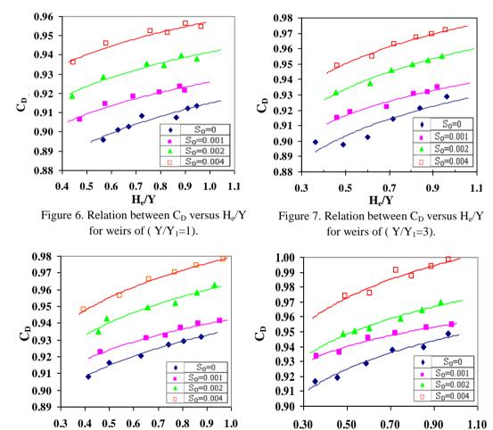
$H_e/Y$ Figure 8. Relation between C<sub>D</sub> versus  $H_e/Y$ for weirs of ( Y/Y<sub>1</sub>=1.5).
