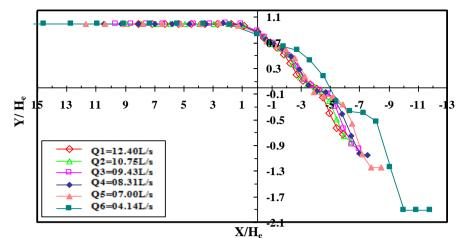
Figure 3. Relation between Y/He versus X/H<sub>e</sub> for all runs of weir  $(Y/Y_1=1.5 \text{ and } S_0=0.001)$
