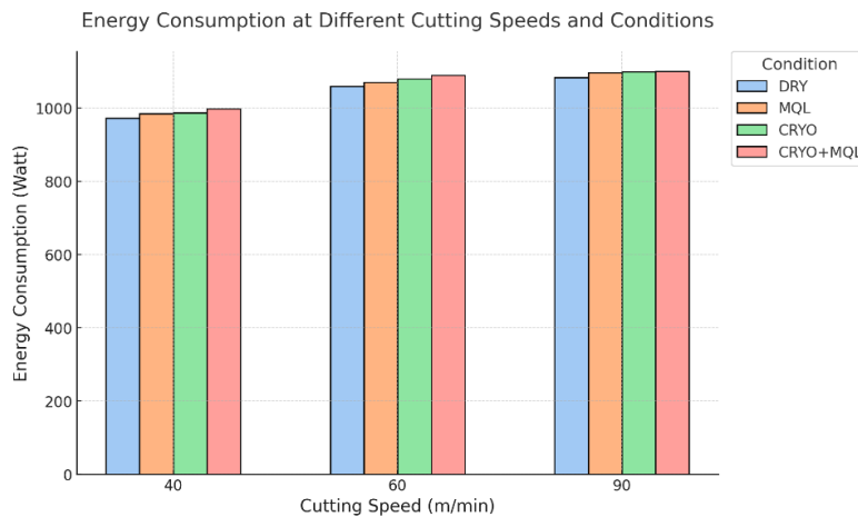
Figure 3.1. Energy consumption values in four different cutting conditions
