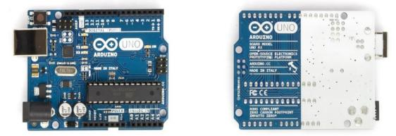
Figure 2. Arduino Uno microprocessor card
