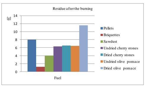
Figure 3. The residue after the burning of solid fuels
