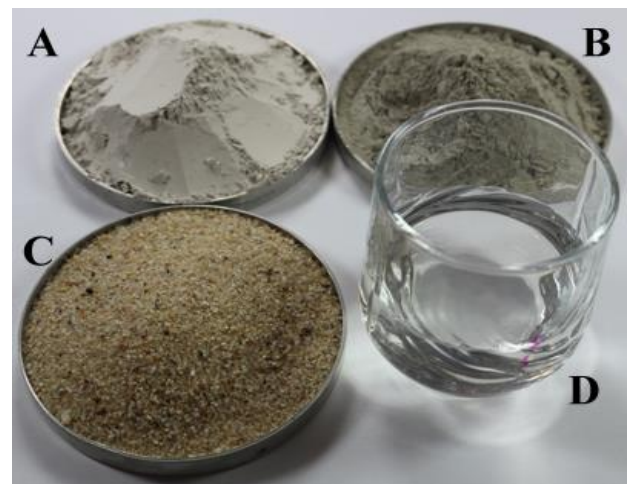
Figure 1. A) Ground Granulated Blast Furnace Slag (GGBFS) B) CEM III/A (S) 32.5 N Blast Furnace Slag Cement C) Silica Sand D) Activator
