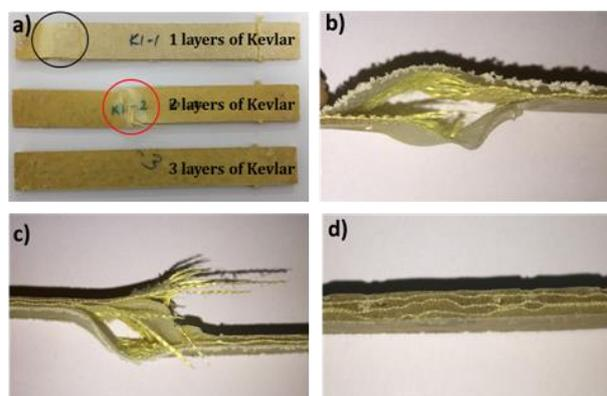
**Figure 2.** Photograph of fractured samples including (a) Top view of tensile test samples, (b) Cross section of 1 layers of Kevlar (black circled area at Fig. 2a), (c) Cross section of 2 layers of Kevlar (red circled area at Fig. 2a), (d) Cross section of 3 layers of Kevlar
