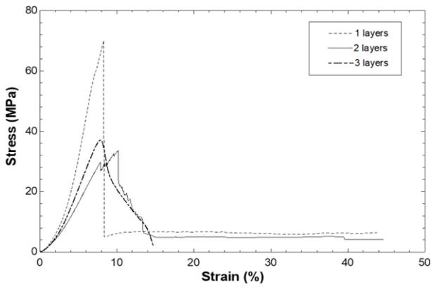
**Figure 3.** Engineering stress – strain curve of 3 different ply number of Kevlar reinforced TPU composites
