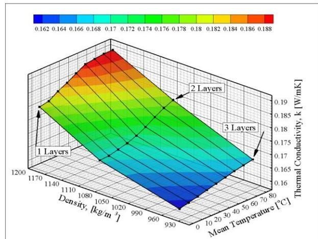
**Figure 5.** Relation between temperature, density and thermal conductivity of various layered Aramid fiber reinforced TPU composites
