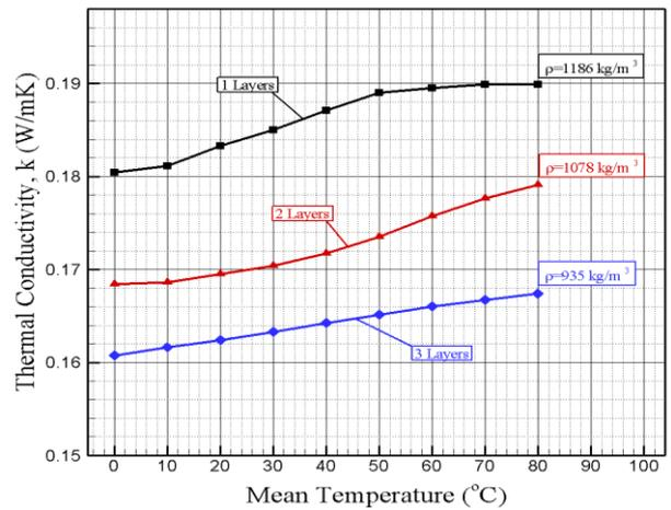
**Figure 4.** Thermal conductivity coefficients of 3 different ply number of Kevlar reinforced TPU composites with different density values depending on temperature
