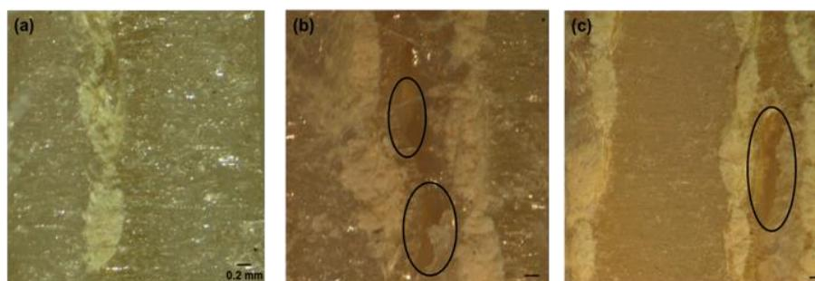
**Figure 1.** Optical image of thermoplastic polyurethane elastomer composite containing (a) 1 layers of Kevlar, (b) 2 layers of Kevlar and (c) 3 layers of Kevlar showing their macroporosity (circled area). Scale bar is set as 0.2mm for all samples.
