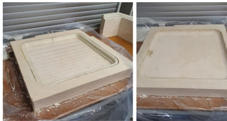
Figure 3. The 3D printed model (left), shown both inside and outside the mould, illustrates its role as an intermediary medium in the fabrication process rather than a finished tabletop.
