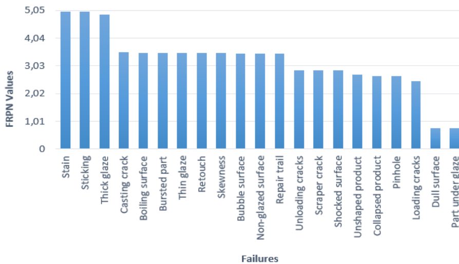
Figure 11. Failure types and FRPN values.
