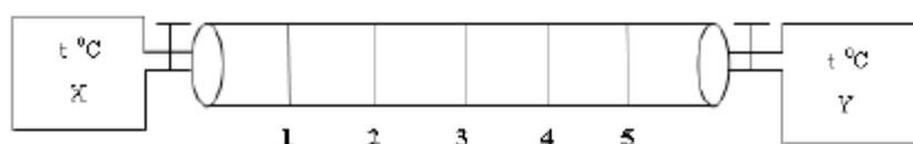
As shown in figure, X and Y gases are left to diffuse toward each other and as they come across at the 5th section of the tube,
