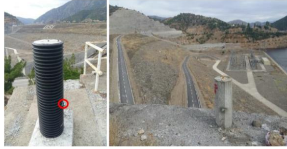
Figure 2. The new reference point N1 (left) and existing observation point N5 (right). Apparatus is shown inside the red circles for precise leveling.
