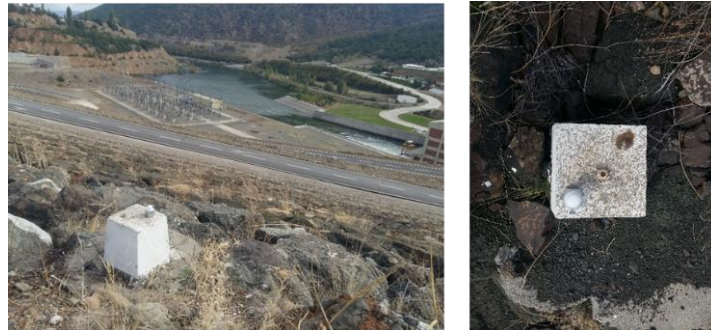
Figure 4. One of the object's points the downstream (left). The white apparatus was used for GNSS and distance observations, while the other add-on (upper right corner) was used for precise leveling.
