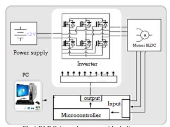
Fig.1 BLDC three phase motor block diagram
