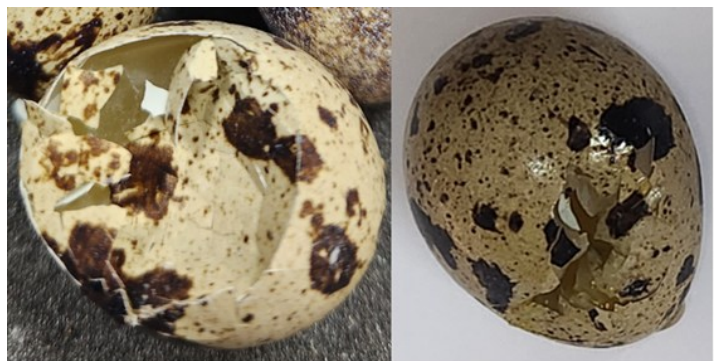
Figure 7. Open large fracture starting from the equatorial region and spreading to the blunt end
