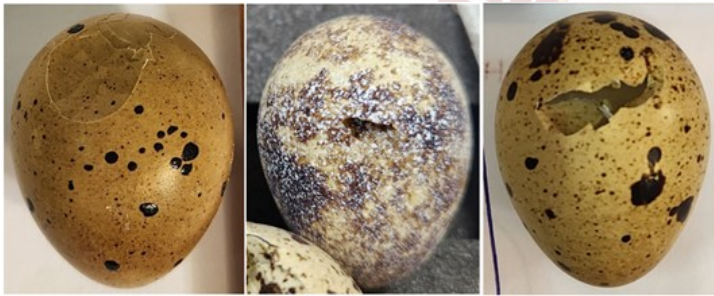
Figure 10. Superficial crack and deep fracture near the equatorial region of the blunt end
