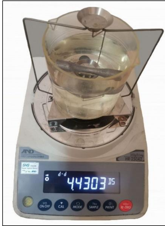
Figure 1: Density measurement equipment (A&D HR-250AZ) and sample orientation for Archimedes method.
