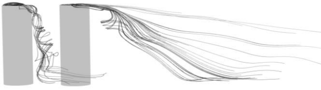
Figure 12. Trailing vortex streamlines for S/D=1 .
