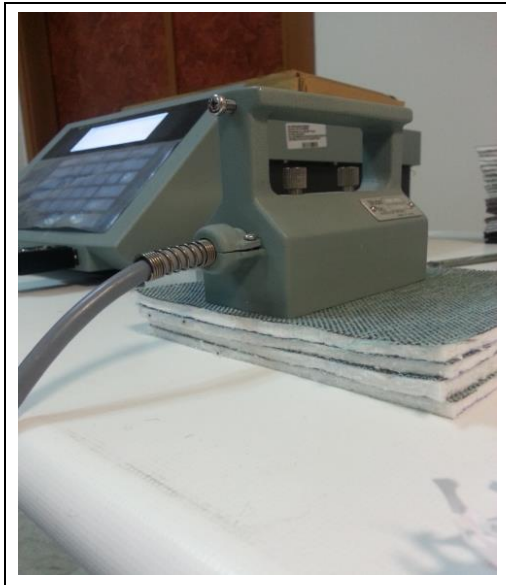
Figure 3. Position of laminated fabrics under the test equipment, Kyoto Electronics QTM-500.
