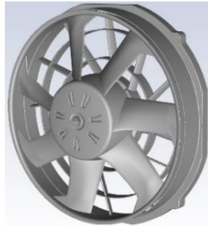
Figure 1. Geometry of an axial-flow fan.
