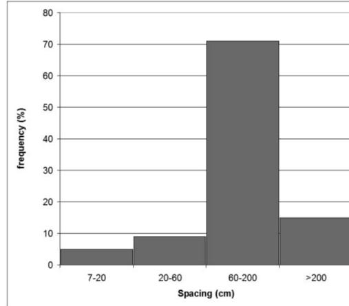
Figure 6. Discontinuity spacing histogram.
