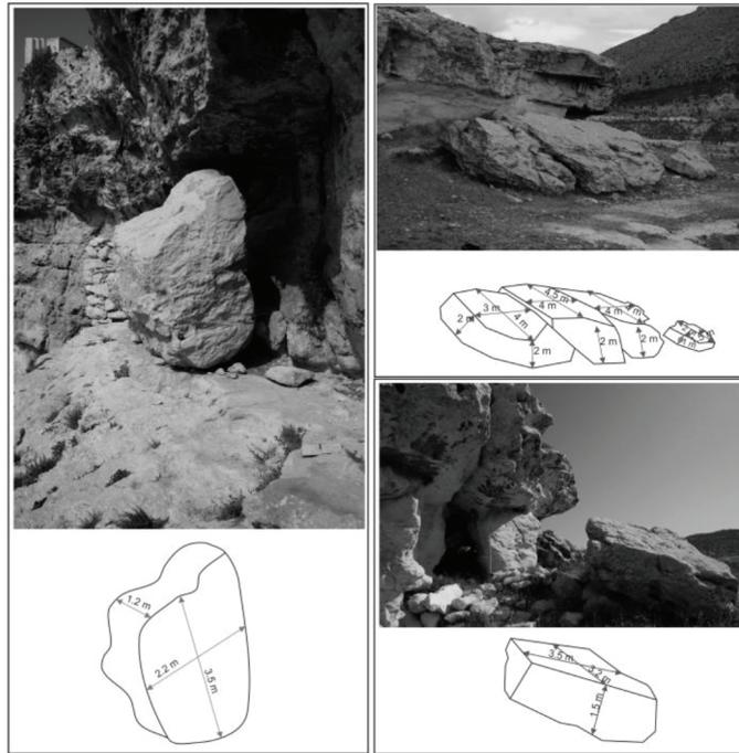
Figure 8. Dimensions of fallen blocks.
