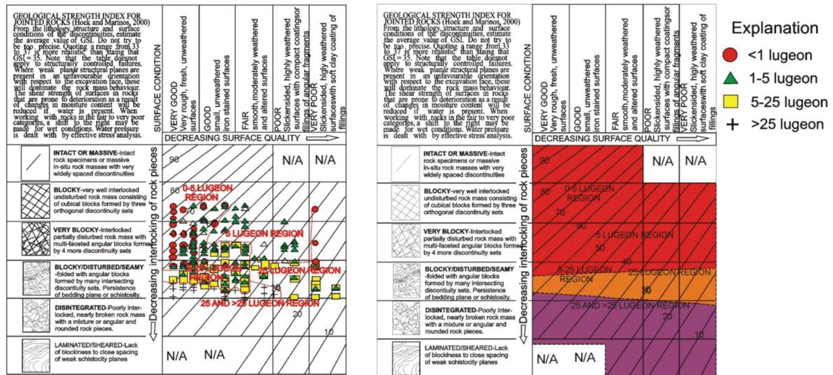
Figure 6a). Coinciding lugeon test results of the study sites on GSI chart b) Determined permeability regions on GSI chart.
