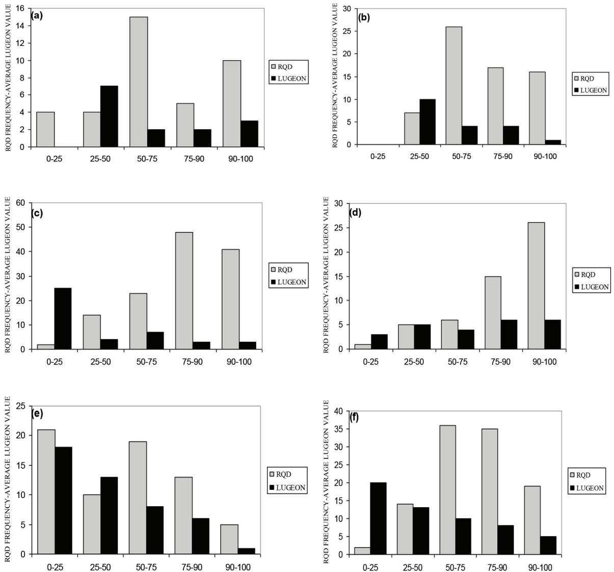
Figure 3. Distribution histograms of RQD-Average results of lugeon tests a) Çan coal mine, b) Laleli dam site, c) Altıparmak dam site, d) İspir dam site, e) Deriner dam site, f) Arkun dam site.
