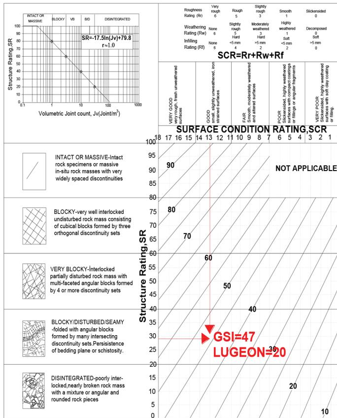
Figure 4. An example about coinciding GSI and Lugeon values on Quantitative GSI chart.
