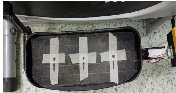
Figure 5. Local Measurement Locations on the Pedal
