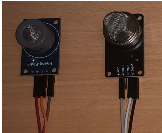
Figure 6. CO and NO x gas sensors used in the study
