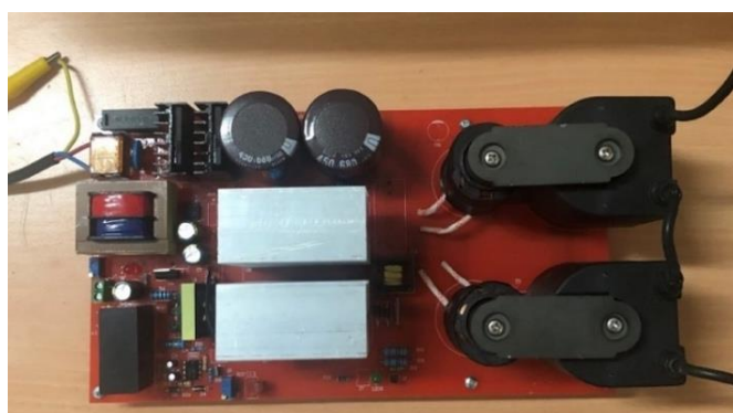
Figure 9. High voltage power supply
