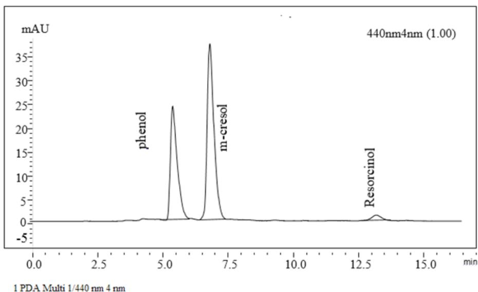
**Figure 6.** Reversed-phase HPLC-UV-vis. chromatograms of quinoneimine derivatives of phenols. Phenol, 6.0 ng; m-cresol, 7.4 ng; resorcinol, 2.0 ng. Column: GL Science Inertsil C<sub>18</sub> RP (5 $\mu\text{m}$ , 250mm x 4.6 mm ID). Mobil phase: acetonitrile-water (45:55%, v/v); Flow-rate: 1.0 mL min<sup>-1</sup>.
