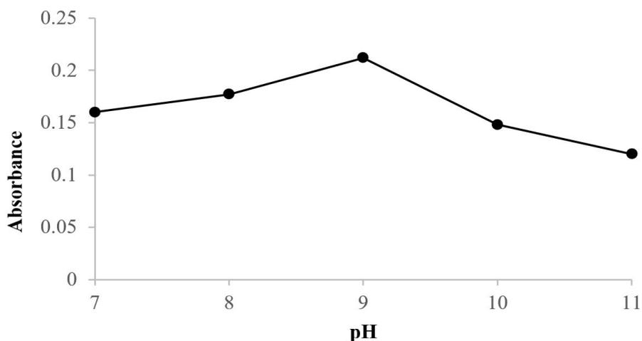
**Figure 2.** Effect of pH on the derivatization reaction between phenol compounds and 4-aminoantipyrine (phenol:  $1 \times 10^{-4}$  M; peroxydisulfate:  $5 \times 10^{-4}$  M; 4-aminoantipyrine:  $5 \times 10^{-4}$  M).
