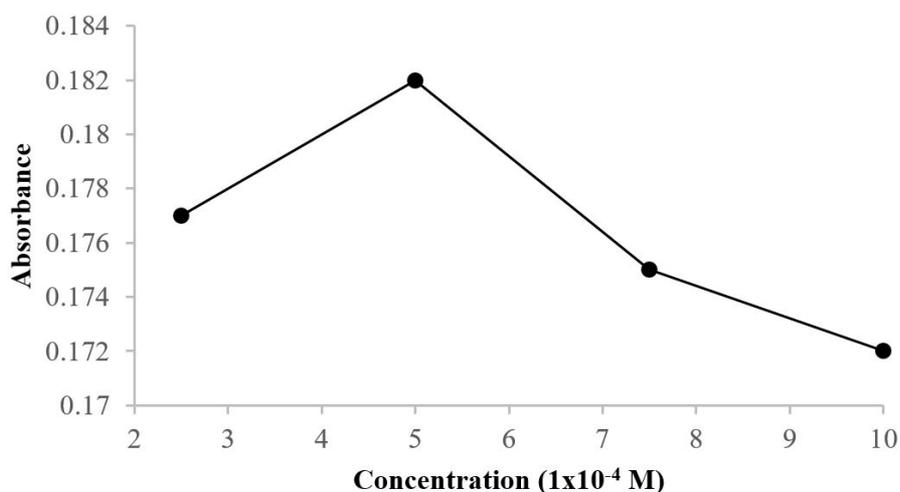
**Figure 4.** Effect of peroxydisulfate concentration on derivatization reaction (phenol:  $1 \times 10^{-4}$  M; 4-aminoantipyrine:  $5 \times 10^{-4}$  M).
