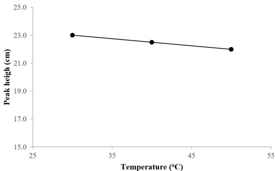
**Figure 5.** Effect of temperature on peak height.
