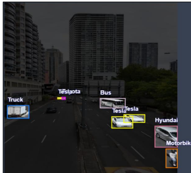
Figure 2. Example of vehicle annotation with bounding boxes and class labels
