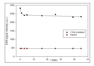
**Figure 7.** Room temperature kinetic behavior of g=2.0047 signal for natural and 5 kGy irradiated samples.
