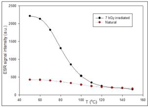
**Figure 6.** Isochronal annealing curve of g=2.0047 signal for natural and irradiated samples between T=50 °C and T=150 °C temperatures.
