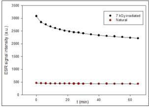
Figure 5. Isothermal annealing curve of g=2.0047 signal for natural and irradiated samples at T=50 °C constant temperature.
