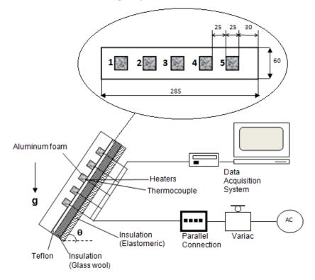
Figure 1.Schematicdiagram of the experimental set-up, heat source layout and assembly (measures are in mm).
