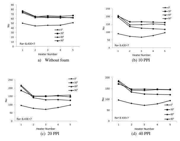
**Figure 4.** Effect of channel inclination angle on Nusselt number for  $Ra = 8.43 \times 10^{7}(a)$  without foam, (b)10 PPI,(c)20 PPI,(d)40 PPI
