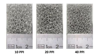
Figure 3. Pictures of aluminum foam heat sinks with various PPI values.
