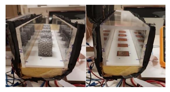
Figure 2. The view of the test section with and without foam case (only copper plate).
