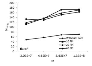
Figure 6. Variation of mean Nusselt numbers according to different Rayleigh numbers in case of channel inclination angle of  $30^{\circ}$
