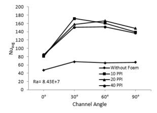
**Figure 5.** Effect of channel inclination angle on the average Nusselt number with and without foam heat sink for Ra= 8.43x10<sup>7</sup>.
