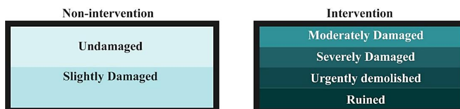
Figure 2: Damage Assessment Classification (Created by the authors)
