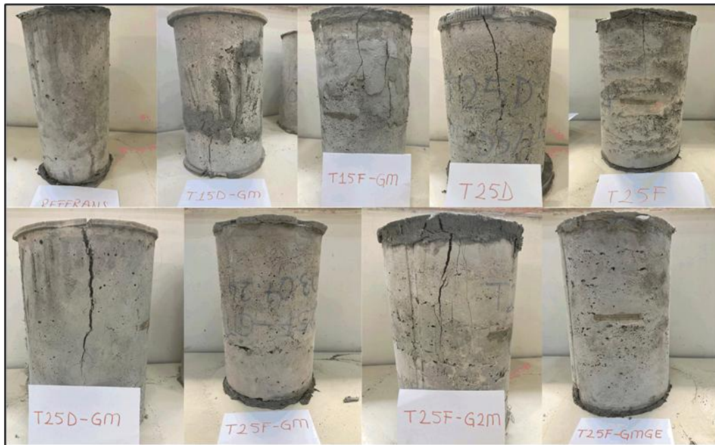
Figure 4. The failure modes of the specimens in different test groups
