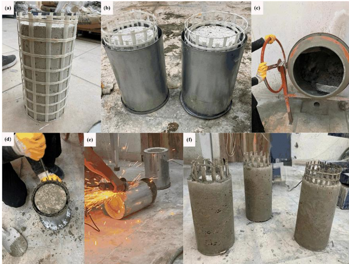
Figure 1. Preparation of the concrete specimens
