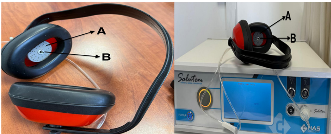
Figure 3. A: Destructor outlet B: Inlet
