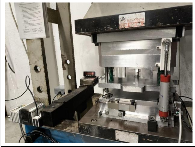
Figure 1. Hydraulic press for deep drawing.
