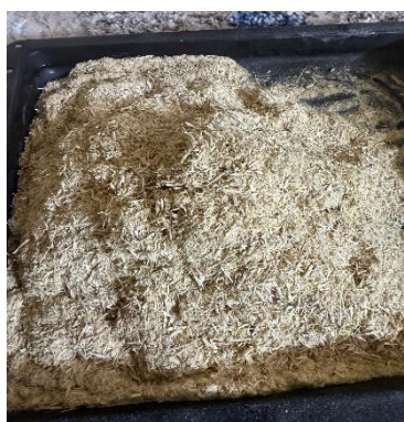
Grinding and washing stage of the Phragmites australis plant
