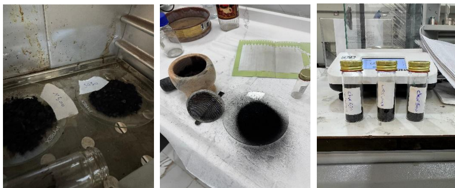
Figure 4: Stages of obtaining activated carbon from Phragmites australis and water hyacinth
