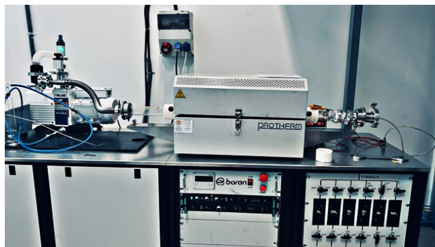
Figure 1. LPCVD system used for the h-BN growth.
