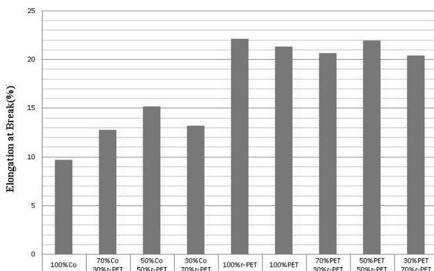
Figure 2. Elongation at break results of the yarns
