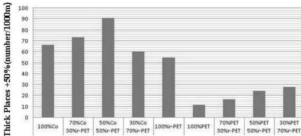
Figure 5. Thick places results of the yarns
