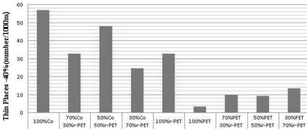
Figure 4. Thin places results of the yarns
