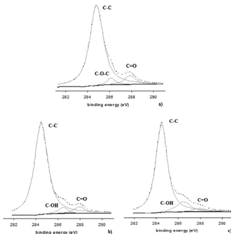
**Figure 2.** Curve fitting of C<sub>1s</sub> peak in C spectra of untreated and enzyme treated PET fabrics [a] Untreated, b) Cutinase treated, c) Lipase treated]
