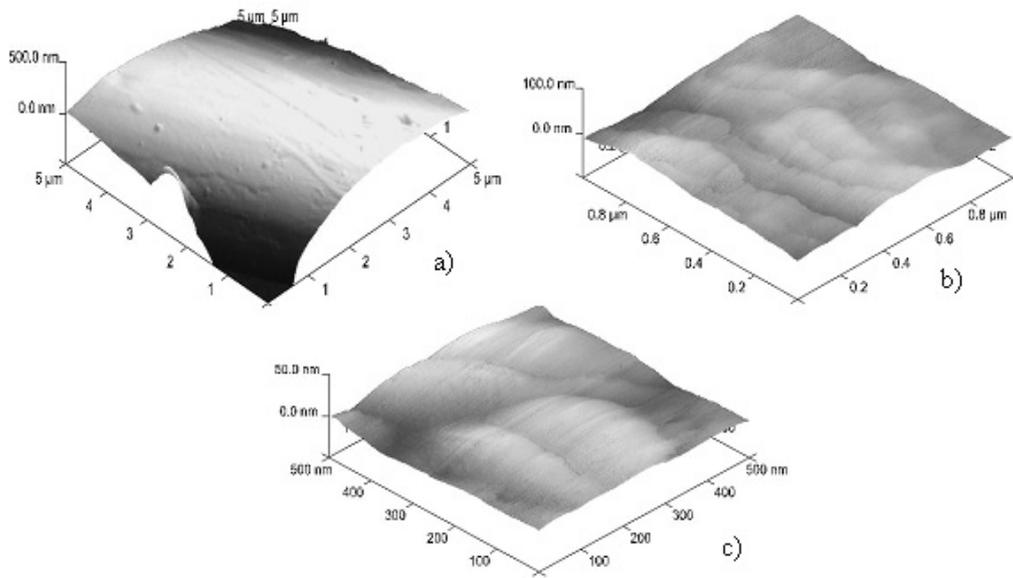
**Figure 4.** AFM micrographs of untreated fabric
