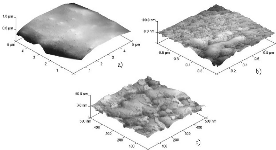
**Figure 5.** AFM micrographs of cutinase treated fabric
