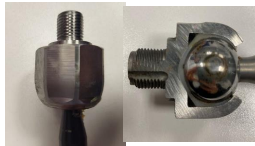
Figure 1. Formed inner tie-rod end stud
