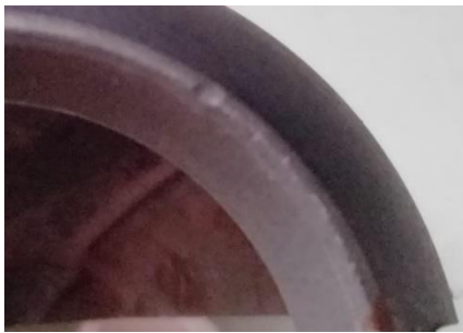
Figure 15. Forming-induced plastic deformation in the tie-rod end formed section
