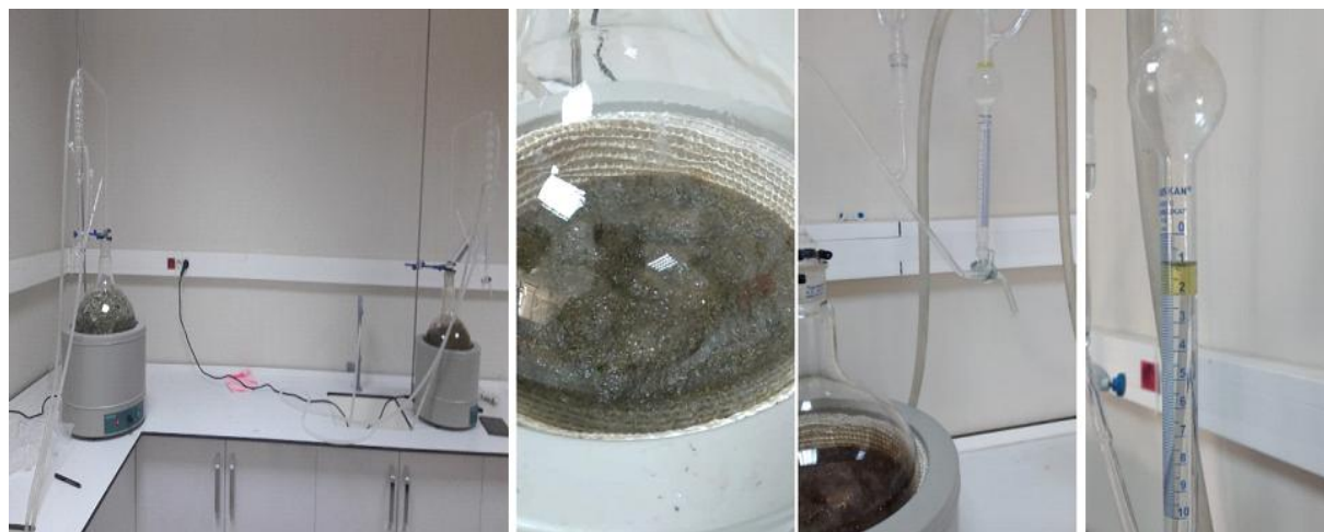
Figure 2. Isolation of essential oils with clavenger apparatus device
