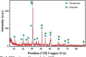
Fig 1. XRD pattern of borax sludge [18]
