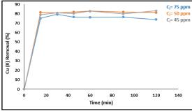
Fig 3. Removal percentage of Cu (II) ions for different contact times
