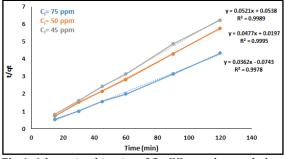
**Fig 4.** Adsorption kinetics of Cu (II) onto borax sludge for pseudo second-order kinetic model
