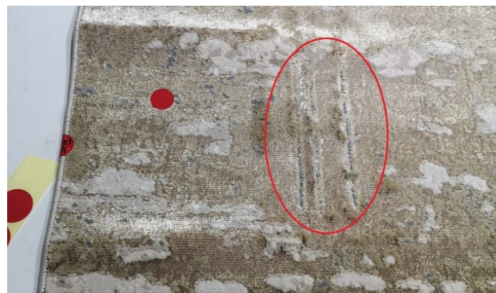
Figure 2. Photographic view of scrape failure [19]
