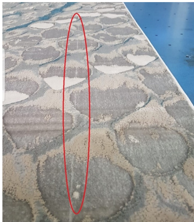
Figure 4. Photographic view of abrage failure
