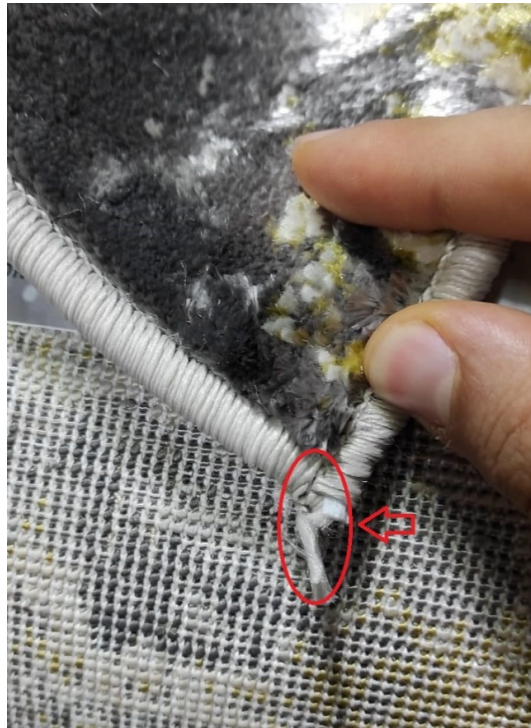
Figure 3. Photographic view of corner burning failure [19]
