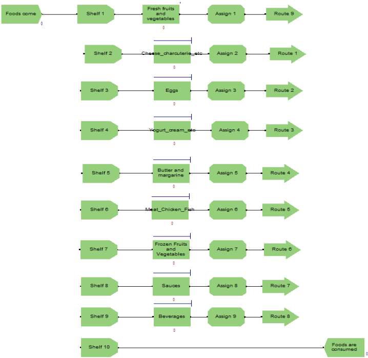
Figure 2. Simulation of Food Placement and Retrieval in a 10-Shelf Refrigerator Using Beta Distribution, represents typical user behavior for product allocation and shelf access within a one-day cycle.
