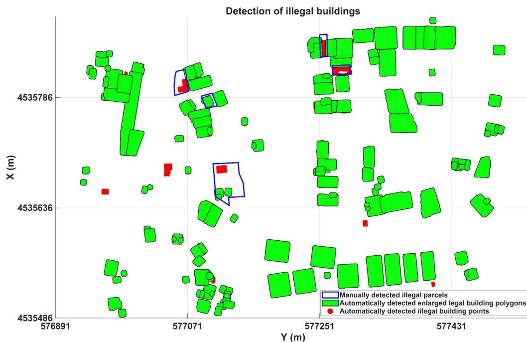
Figure 11. The visualization of automatically detected illegal structures (red), legal buildings (green), and parcels containing illegal buildings identified manually by the municipality (blue).
