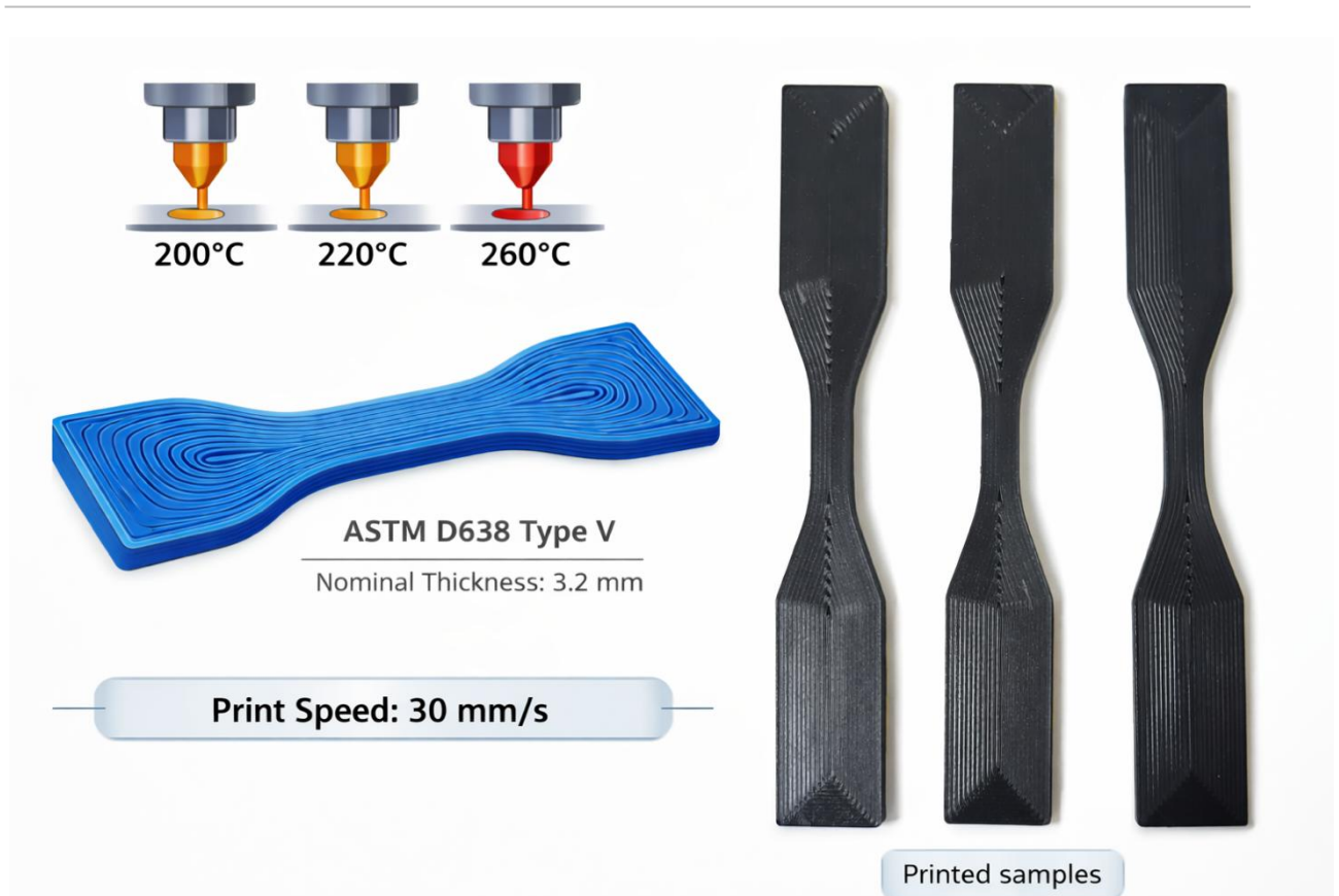
Figure 4 Scheme of printing parameters and infill type and printed specimens
