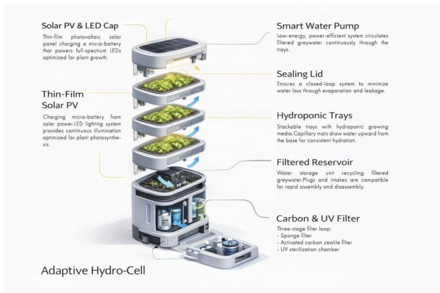
Figure 4. System Diagram of the Adaptive Hydro-Cell. Schematic showing airflow, water recirculation, lighting array, and modular connectivity.
